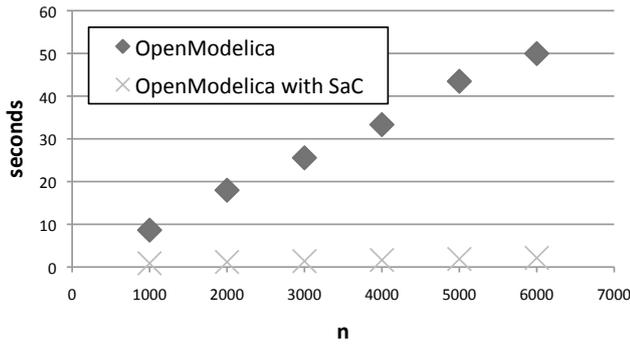
**Figure 2.** The WaveEquationSample run for different number of sections ( $n$ ) with functionODE and Euler loop implemented as pure OpenModelica-generated C++ code and as OpenModelica-generated C++ code with function-ODE and Euler loop implemented in SAC. Start time 0.0, stop time 100.0, step size 0.002 and without CUDA.
