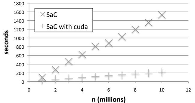
**Figure 5.** WaveEquationSample state derivative calculations embedded with an Euler loop, both written entirely in SAC, run sequentially and with CUDA for varying number of sections ( $n$ ). Start time 0.0, stop time 100.0 and step size 0.002.
