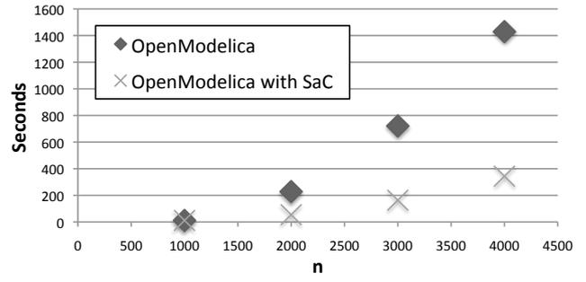
**Figure 1.** The WaveEquationSample run for different number of sections (`n`) with `functionODE` implemented as pure OpenModelica-generated C++ code and as OpenModelica-generated C++ code with `functionODE` implemented in SAC. Start time 0.0, stop time 1.0, step size 0.002 and without CUDA.
